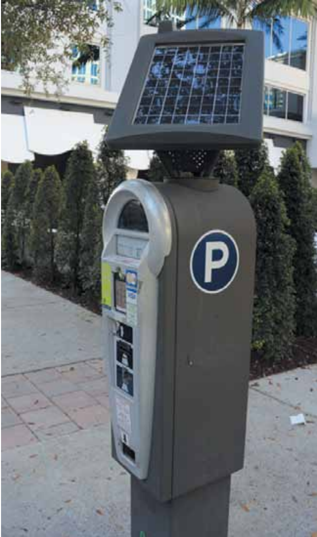
The solar panel on top powers this parking meter.
